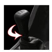
Install the new shift knob to the desired location and lock in place with supplied set screw and allen key.
