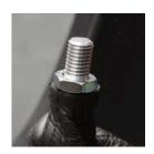
3. Screw in supplied set screw plug into the unused opening.
