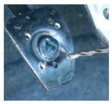
3. Fasten the pedal covers using the supplied stainless screws.
