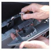
Window switch removed from switch plate.
