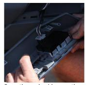
From the underside snap the window switch into the billet switch plate.
