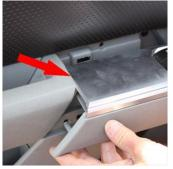
Line up the round alignment tabs at the bottom of the arm rest pad and press back into place.
