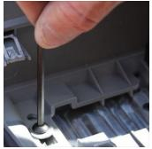
Using the supplied hardware tighten down the switch plate to the lower arm rest. Do not over tighten.
