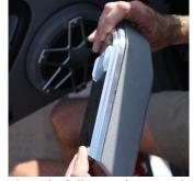
Place the billet window switch plate on top of the lower arm rest pad as shown and align it properly.
