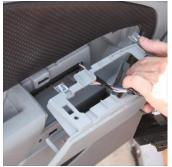
Grasp the lower part of the arm rest and pull away from the door panel as shown.
