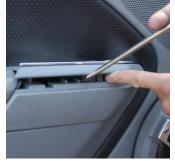
The top plate will separate from the bottom piece as shown.
