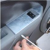
Using a smooth flat headed screw driver gently pry up on the plastic switch plate. There are two clips holding it place.
