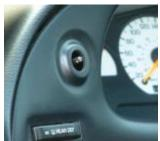
Using a #20 Torx screwdriver, remove the two retaining screws. Remove the outer gauge bezel by gently pulling on the outside edges. It will "pop" off.
