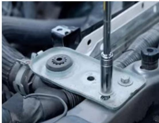
2. Remove [2] 10mm screws holding each radiator mounting bracket and remove the rubber grommets from the brackets. You will re use the grommets.
