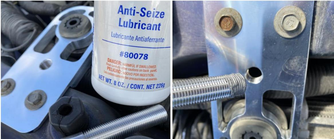
4. Attach the UPR radiator mounts using the factory 10mm screws (see picture 4A). **Apply anti-seize to the aluminum hood pins** and thread them into the radiator mounts. Fasten the hood pins to the radiator brackets using the nuts. Pin height will be adjusted later.
