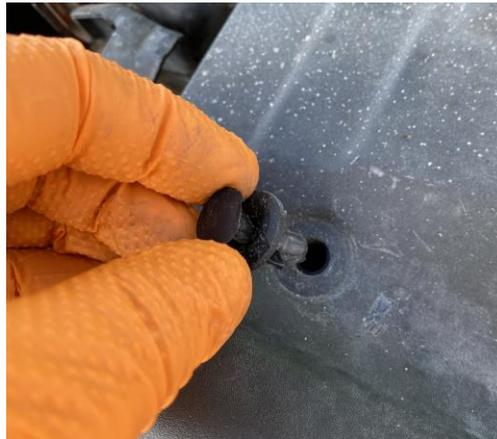
1. Remove the plastic pins holding the black plastic radiator cover and remove the cover.
