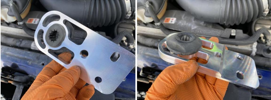
3. Insert the rubber grommets into the new billet aluminum radiator mounts.
