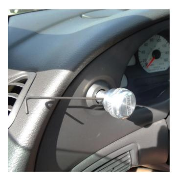
3. Now remove the factory gauge bezel from the dash board.
