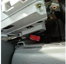
8. Now remove the gauges from your mustang and work on them on a counter top.9. Unscrew all the gold screws and gently lift the plastic gauge face off the speedo gauges.
