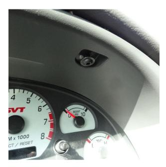
2. Use an allen wrench or flat head screw driver to remove the factory headlight knob.
