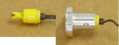
**<u>Type A</u>** dip stick handle. This style is made of metal and is most common on the fox body (87-93) Mustangs. Remove the area highlighted above with a grinding wheel or hacksaw. Do not cut below the dimple in the side of the shaft. View of the modified factory dip stick handle. Note the location of the cut and that some of the dimple is still remaining. Slide the dip stick cover over the factory handle shaft. Install provided set screw and tighten.
