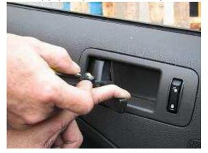
4. The cover in the door pull/armrest needs to be pried away, and the T30 torx screw behind it removed
