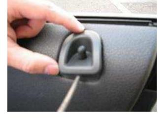
7. Using the 6mm socket, remove the (9) nine screws on the periphery of the door and the one hidden in the window switch area. See figure below for screw locations.
