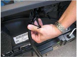
11. Remove the cable and the spring inside the stock handle. Remember the orientation of the spring, which will be re-used with the new handle.
