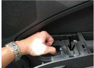
6. Remove the door lock bezel by slightly lifting it up (a small screwdriver may be needed)
