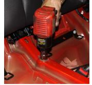
Install either the factory bolt on the 05-10 Mustangs or use the provided bolt/washer on the 2011 Mustang. Once tight reinstall the back seat.
