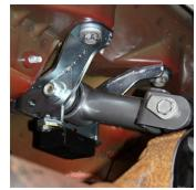
Align the rear end with the upper control arm and install with factory hardware. Using a jack under the rear end will help line this up. Tighten all bolts.
