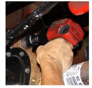
Next remove the back bolt holding the stock control arm to the rear end housing and remove the upper control arm/mount assembly.
