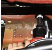
Under the car remove the two bolts holding the 3<sup>rd</sup> member to the bottom of the car.
