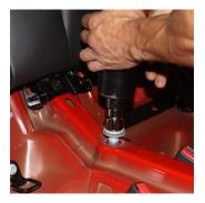
Remove the lower portion of the back seat of your car exposing the top bolt for the third member. Remove this bolt.
