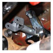
Install the upper control arm into the new 3<sup>rd</sup> member mount with the thick billet spacers on either side of the control arm and secure with provided nut, bolt and washers. Install the pinion snubber to the 3<sup>rd</sup> member then put assembly into place.
