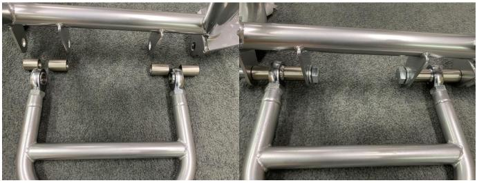
Arrange the sleeves so that the short ones are towards the front of the car. Install the factory A arm bolts or use UPR's 79-04 Heavy Duty A arm hardware kit 2025-45 (included in UPR's Heavy Duty K member and A arm hardware kit 2025-07). Tighten the A arm hardware just until any slack between the K frame tabs and A arm sleeves is taken up, then hand tighten to snug. Do not overtighten.
