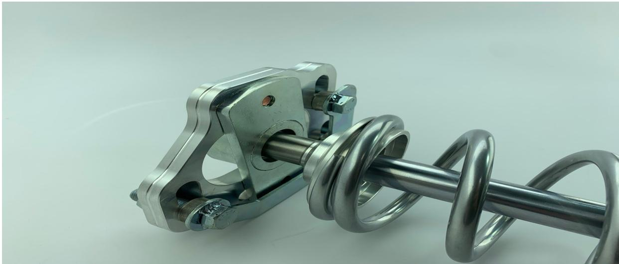
**Step 8:** There will be two different spacers that will slide over the top of the struts stud. Depending on how much of the strut's stud is sticking out determines which spacer to use.
