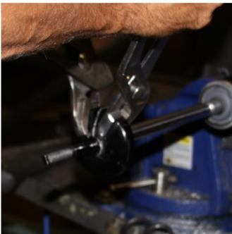
Using two sets of pliers work the shield apart until you can remove it from the shaft of the shock. Another option would be to cut the shield on the side as we did we step 3.
