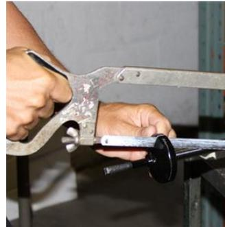
Next make a cut in the metal dust shield with a hack saw or cut off wheel.
