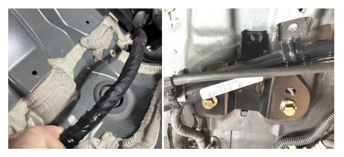
7. Some cars will have more seam sealer in the trunk area than others. It is recommended to remove the factory sealer as it will be hard enough to interfere with properly aligning the retainer plate. We used the retainer plate to mock up and see where we needed to scrape the sealer off.
