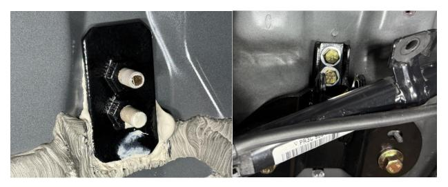
9. Before installing the shock, assemble the upper shock eyelet conversion. If you are using a factory or aftermarket shock bump stop, slide it onto the shock shaft. Install the thick washer, then the nut, then the rod end and tighten it. (this kit is designed for shocks using M10 1.5 thread only)
