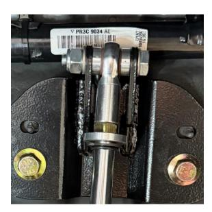
11. Reinstall the lower portion of the shock into the lower control arm. The 15mm lower shock bolts should be torqued to 35 ftlbs.
