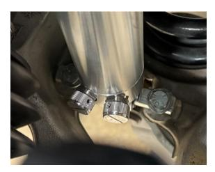
12. Reinstall the trunk liners. Reinstall the wheels. The UPR upper shock mount moves the upper shock mounting point up ¾ of an inch. This helps to correct the shock length on lowered cars and will increase bump travel.
