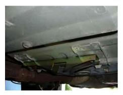
Line up the rear torque box reinforcements, there is a left and right. As seen above prep the surface for welding by removing all paint with either sand paper or 3m sanding wheel. Hold reinforcement in place and weld along the edges.
