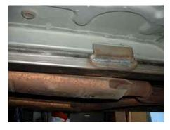
Line up the subframe connector to the frame rails and mark off the welding points around the plates. Clean off any paint along those points for a good weld. Place the subframe back into place and support with floor jack so it's good and tight and weld into place. Using C clamps to keep it aligned to the front and rear may be necessary.
