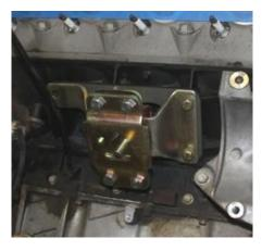
Using the M10-25mm bolts and lock washers align the front 2 bolt holes with the 4.6 motor mount and the adapter plate and thread into the block. Do not tighten these all the way.
