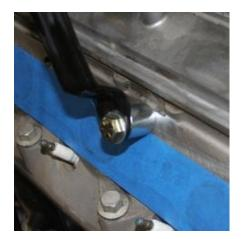
Place the provided 7/8" spacer between the dipstick tube bracket and the cylinder head and put the M10-35mm bolt and washer through the bracket and spacer and tighten. Note: it is possible to bend the dipstick tube and bracket to clear the motor mount if clearances are tighten.
