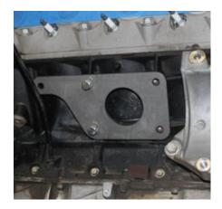
Place the plate against the factory mounting location with the arm of the plate facing the back of the engine as shown above. Using the M10-20mm long bolts and lock washers thread the bolts in by hand into the center two holes. Do not tighten yet.
