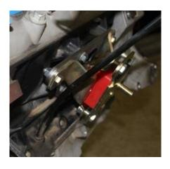
Use a supplied M10-25mm hex bolt and flat washer to go through the arm of the 4.6 motor mount and the adapter plate and secure with a nylock nut and tighten.
