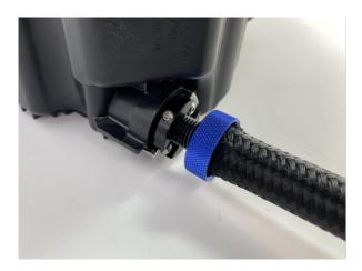
Once all of the oil is drained, rotate the body of the drain plug counter clockwise to remove it from the oil pan.
