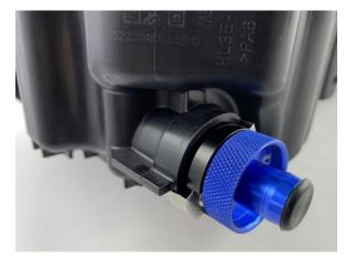
Wipe out any oil residue from the drain hole.
