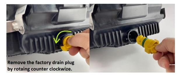
Remove the factory drain plug by rotating the plug counter clockwise.
