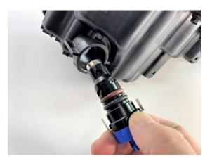
Wipe out any oil residue from the drain hole, and wipe off and clean the oil drain plug.
