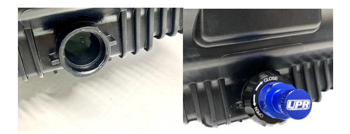
5. When the oil is drained completely, wipe out the oil pan drain hole, and wipe excess oil off the drain valve. Make sure the drain valve in is the fully CLOSED position by rotating the blue valve clockwise.
