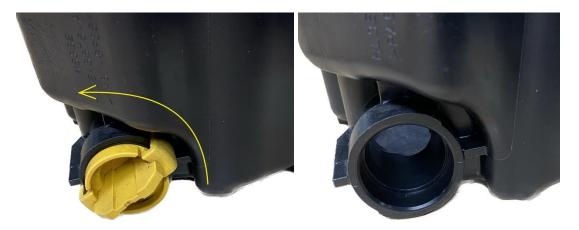
1. Be sure the engine is cool, and you have a proper oil drain pan in place before removing the drain plug. Remove the factory drain plug by rotating the yellow plug counter clockwise. Once the oil has drained *completely*, wipe out the drain hole to remove residual oil.
