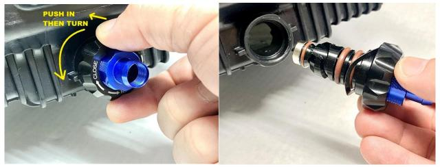
**4.** When the oil is drained, remove the drain valve to allow all of the remaining oil to drain out. **Push the drain valve in towards the oil pan firmly before turning** the black portion of the drain plug counter clockwise. Failure to push the drain valve body in towards the oil pan and / or using a wrench or other tools to turn the drain valve will result in oil pan damage.
