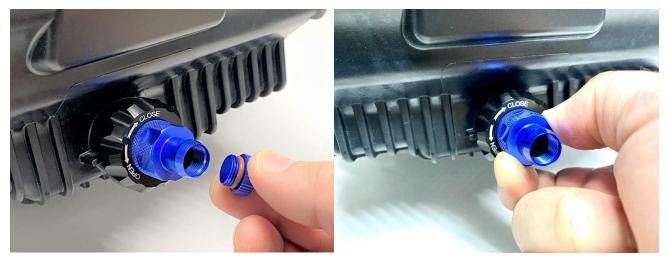
**3.** To use the drain valve to remove engine oil, remove the billet dust cap by rotating counter clockwise. You can slide a 1/2" hose (not included) over the barbed end of the drain valve to control oil flow into a drain bucket if you like. Turn the blue valve counter clockwise to allow oil to flow out.
