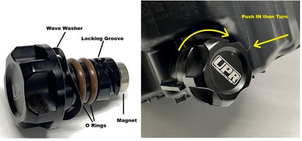
2. To install the UPR Billet Oil Drain Plug, be sure the wave washer is in place and insert the drain valve so that the grooves engage the tabs inside the oil pan drain hole. Push in firmly then rotate the drain plug clockwise until it stops. You will feel the drain valve body engage and lock in. If you have the grooves in the valve lined up with the tangs in the oil pan, it will turn easily. If it is difficult to turn, stop, and recheck the alignment to prevent damage to the oil pan
