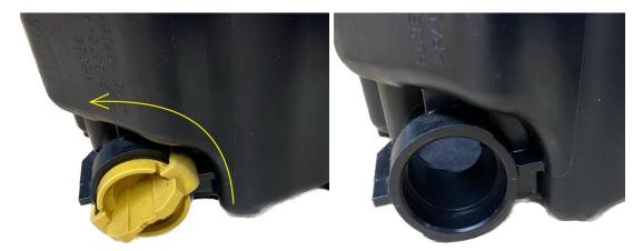
Be sure the engine is cool, and you have a proper oil drain pan in place before removing the drain plug. Remove the factory drain plug by rotating the yellow plug counter clockwise. Once the oil has drained *completely*, wipe out the drain hole to remove residual oil.
