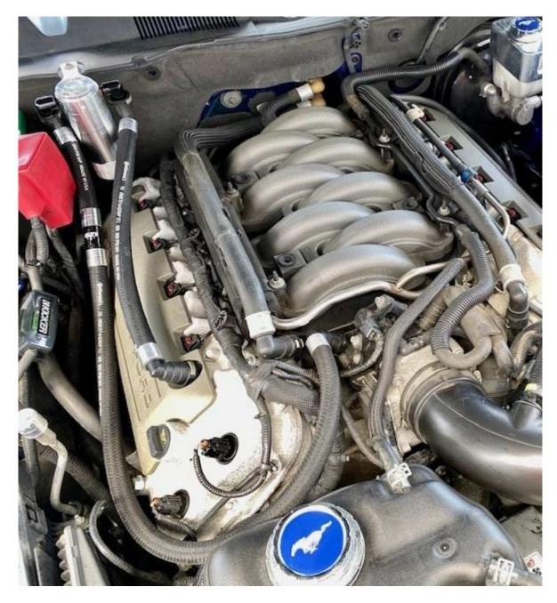
**3.** Remove the factory PCV hose. Install the shorter hose in the kit. It will connect from the PCV valve to the right side of the catch can. Install the longer hose connecting it from the left side of the catch can to the intake manifold vacuum fitting. If you selected to add the check valve, the arrow on the check valve must face away from the catch can, towards the engine.
