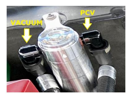
2. The fitting closest to the engine will connect to the PCV valve on the passenger valve cover. The fitting closest to the battery will connect to the vacuum fitting on the intake manifold.
