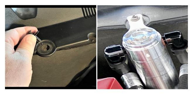
1. Mount the catch can to the passenger side of the fire wall near the battery. You will remove one of the factory plastic retaining pins and use the supplied hardware to secure the catch can.
