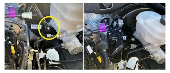
4. The clean side catch can will mount to the Brake Master Cylinder stud. Remove the nut with a 13mm wrench, install the UPR Billet Flat Bracket onto the stud, adjust the can and bracket, and reinstall the nut.
