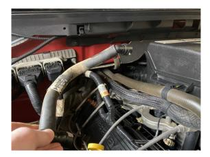
Locate the factory PCV hose that runs from the PCV value on the passenger value cover to the vacuum port on the passenger side of the intake manifold and remove it.
