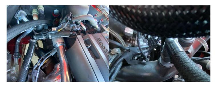
5. Connect the hose to the valve cover and reconnect the VPS harness to the sensor. Connect the other hose in the kit to the air intake tube and route both hoses towards the catch can bracket. Be sure to route the hose avoiding any hot exhaust and secured from any hazards.
