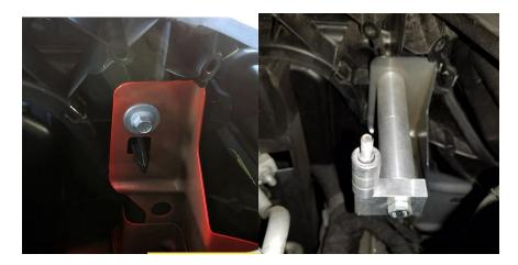
1. Locate the bolt at the radiator support behind the passenger headlight. Remove the bolt and install the UPR Billet bracket as shown.
