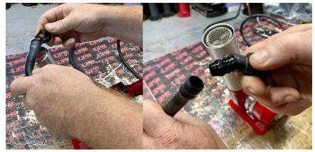
3. Using a heat gun or hot water to warm the factory plastic tube, remove the stock quick disconnect fitting from the tube (end closest to the windshield/VPS sensor). You will re-use this fitting.
