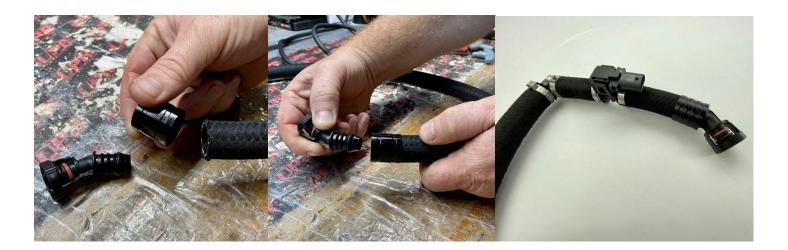
4. Assemble The UPR hose with the VPS on it by sliding the UPR billet hose end on, then inserting the factory fitting into the hose as shown.
