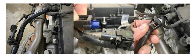
2. Locate the Crankcase Vent (CCV) Tube at the left rear of the valve cover. Disconnect the Vapor Pressure Sensor (VPS) and remove the factory tube assembly by disconnecting the fittings at the valve cover and intake tube fitting. Do not pry the fittings. They are made to release easily by hand.
