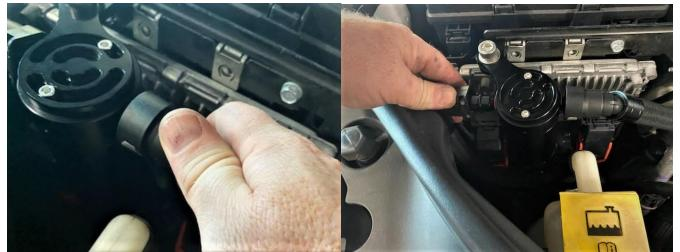
6. Install the UPR Plug N Play<sup>™</sup> Fittings onto the catch can. The 'Dirty' side hose will connect to the left side of the catch can. The 'clean' side hose will connect to the right side of the catch can.
