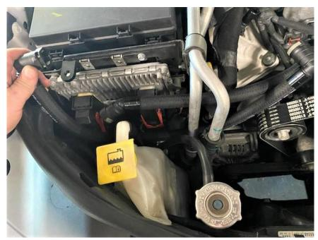
3. The longer of the two hoses in the kit will be the PCV or 'dirty' side hose. The vacuum hose, or 'clean' side hose will be shorter. Route the hoses behind the AC lines as shown. If you selected to add a UPR Check Valve to your catch can kit, it will be installed in the 'clean' hose. Be sure the arrows on the check valve are facing towards the engine when routing the hose.
