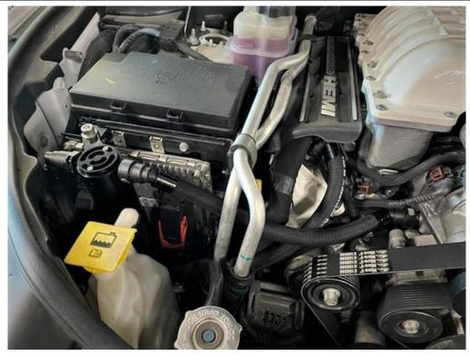
Check your UPR catch can every 500 to 1000 miles at first to get a feel for your engine's needs. You can easily remove the catch can for cleaning and inspection by pressing the grey buttons on the Plug N Play<sup>™</sup> fittings (NEVER PRY THE BUTTONS OUT) to release them, and removing the mounting bolt. The catch can containment cup unscrews so you can dispose of the liquid properly with waste oil. Do not return the liquid to the crankcase.
