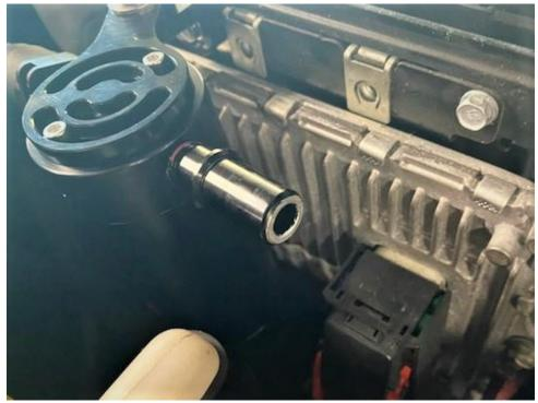
5. Install the UPR catch can onto the 90-degree billet bracket with the supplied bolt. The vacuum or 'clean' side fitting will be marked with a silver ring at the end of the fitting as shown. This side of the catch can will face towards the engine.
