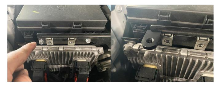
Use a 10mm wrench or socket to remove the left side bolt from the ECU mount. Install the UPR 90-degree billet bracket as shown using the supplied bolt.
