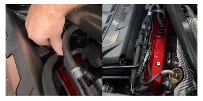
2. The UPR PCV hose will be the shorter of the two in the kit. Install the hose onto the PCV fitting and route it to the rear of the engine as shown. The hose can be secured with the factory looms. The hose end fittings are not crimped, so they can be rotated as needed.
