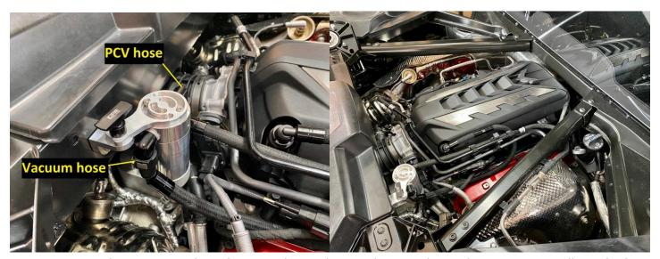
6. Connect the vacuum and PCV hoses to the catch can. The UPR Plug N Play connectors will simply clip on just like the factory connectors. To release them, Push both grey buttons on the fitting and slide it off. The catch can will be easily serviced by disconnecting the Plug N Play fittings, unscrew the catch can from the mount, and dispose of the liquid by unscrewing the containment cup to dump it out. Always dispose of the liquid like you would used oil.
