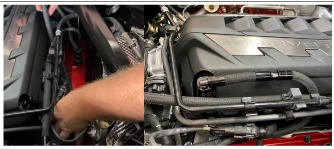
**3.** Route the UPR Vacuum hose behind the PCV and Fuel lines, close to the intake, and loop it towards the rear of the car. The check valve in the hose has an arrow printed on it. The hose must be routed so that the arrow points towards the engine, away from the catch can.
