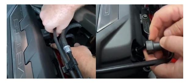
1. Remove the factory PCV hose. The hose runs from the vacuum port on the intake manifold to the PCV fitting at the lower front passenger side of the intake. It is easily released by pushing the buttons on the side of the fitting.
