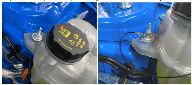
2. Install the Clean Side Catch Can onto the stud and secure it with the supplied knob as shown.
