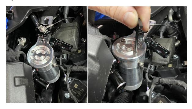
**6.** Locate the factory PCV hose that connects the PCV valve on the passenger side valve cover to the intake manifold/ Supercharger vacuum fitting. Remove the hose by sliding the tabs on the fittings to the side and lift it off.
