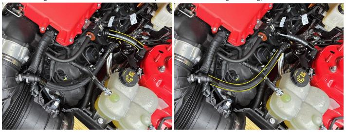
Always check and drain the catch can more often in winter / freezing weather. If the water/oil mixture in the catch can is allowed to freeze it will cause damage to the catch can and internal components. Any damage due to freezing is NOT WARRANTY. You must dispose of the liquid collected in the catch can properly (with used waste oil) properly according to your local laws.
