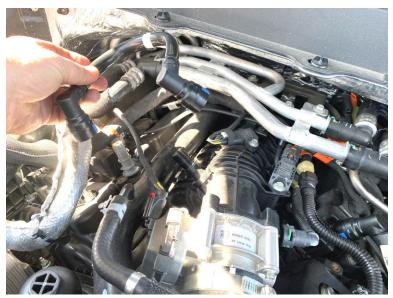
2. Locate the factory PCV hose. It runs from PCV on the passenger valve cover to the intake manifold vacuum port. Remove the hose. Keep the hose in case the vehicle is to be put back to stock.
