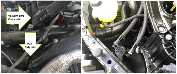
4. Connect the Dirty Side hose from the PCV on the passenger side valve cover to the inlet fitting on the catch can. Route the hoses so they are clear from hazards like belts, fans or exhaust.
