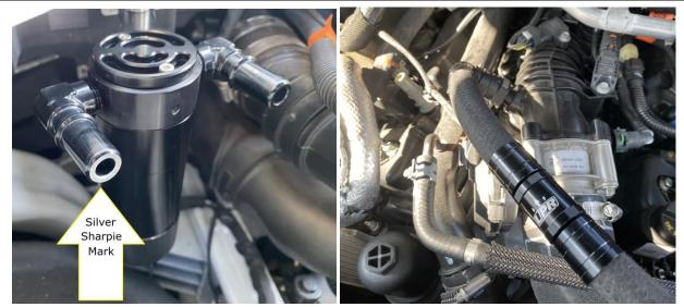
3. The outlet from the catch can will be marked with a silver Sharpie at the end. Install the vacuum hose by connecting from the outlet of the catch can to the intake manifold vacuum port. If you selected the Pro Series Check Valve upgrade, be sure the arrow printed on the check valve faces away from the catch can, towards the engine.
