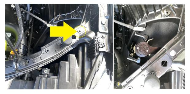
1. Find the un-used factory hole in the radiator support to the right of the hood bumper on the driver side. Mount the catch can with the provided hardware. You will need a 5/32 allen wrench.
