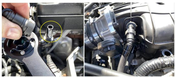
**3.** The outlet fitting on the catch can will have a silver mark on the end. This will connect to the intake manifold. The hose connecting to the manifold will have a check valve in it. Be sure the arrow on the check valve faces away from the catch can, towards the engine. Connect the other side of the catch can to the fitting in the lifter valley. To release the UPR Plug N Play connectors, squeeze both grey buttons, never pry them out.
