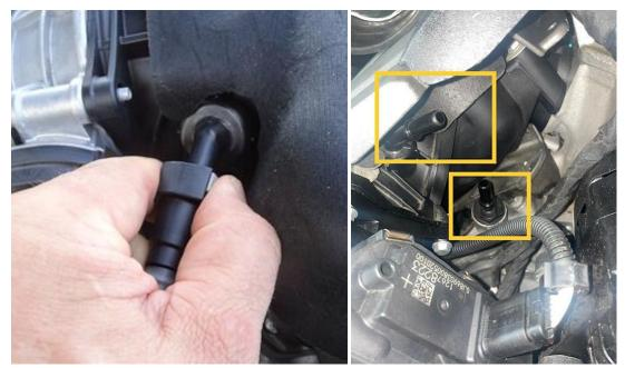
2. Lif the engine cover and locate the Factory PCV hose. It will connect from the intake manifold vacuum fitting, just behind the throttle body on the driver side of the engine to the PCV fitting in the lifter valley plate. Press the buttons on the fittings to remove the hose.
