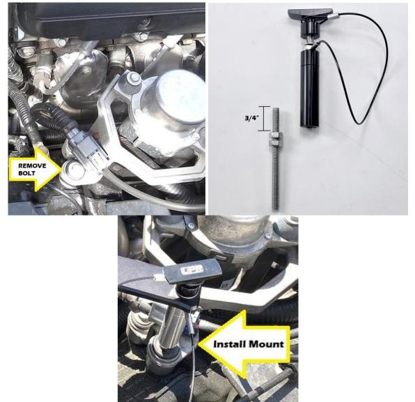
Locate the forward vacuum pump bolt, and use a 10mm socket to remove it. Install the Provided stud in it's place. Leave <sup>3</sup>/<sub>4</sub> of an inch of the stud above the nut. Tighten the lower nut to secure the stud. Screw the round mount onto the stud, then tighten by using the upper nut.
