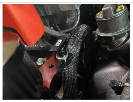
3. Install the UPR Breather Tank onto the mount with the supplied knob and washer. The mount and catch can bracket can be adjusted for the best positioning.
