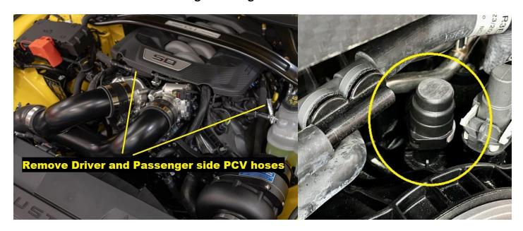
1. Remove the driver and passenger side PCV hoses. Cap the Intake manifold vacuum fitting with the provided cap. Also cap the fitting on the supercharger intake tube with the supplied cap.
