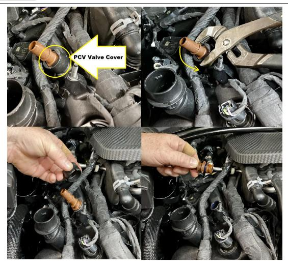
The PCV valve is located on the passenger side valve cover. It is secured with a glued-on cover.
