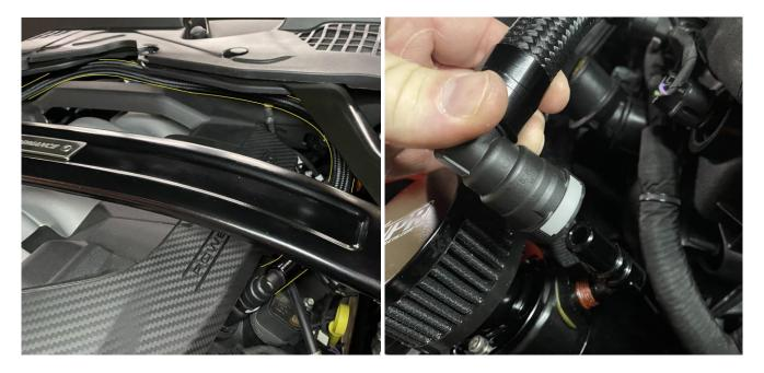
4. Route the longest hose in the kit behind the intake manifold, along the firewall and connect one end to the driver side valve cover. Connect the other end to the breather tank. The UPR Plug N Play™ fittings will click on when fully engaged. To release the fittings, press the grey button on the fitting, never pry or remove the grey buttons.
