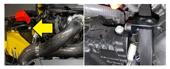
2. Install the UPR Mount onto the passenger side air box bracket with the provided bolt as shown.
