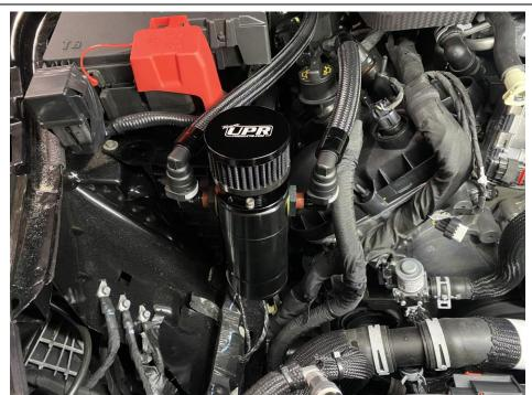
5. Connect the short hose from the passenger side valve cover to the breather tank. Adjust the brackets for the best fit and tighten the brackets.
