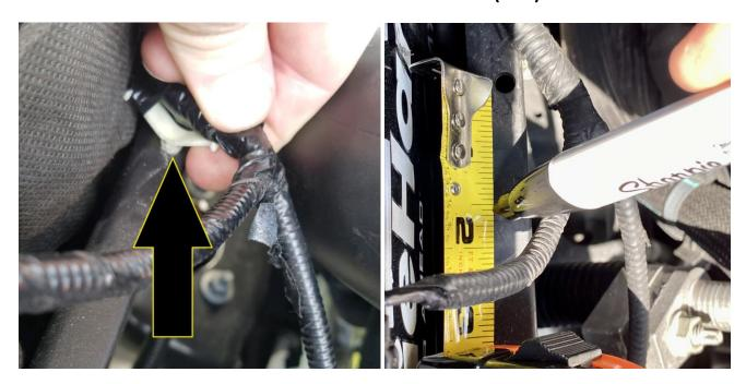
1. The F-150 will have a hole on the battery box lip that is used to secure the positive battery cable with a push clip. Measure 1 and ½ inches forward from the hole and drill a ¼" hole in this location. Using the supplied Mount and hardware, Install square block as shown Overtightening the mount could damage the battery tray.
