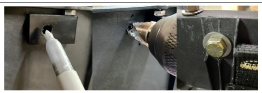
2. \* Optional Step. To increase the stability of the mount, start by marking the location of the hole in the support block, drill a 3/8 hole (this is best done with the battery removed) and install a 3/8-24 bolt from the inside of the battery tray out through the bracket.
