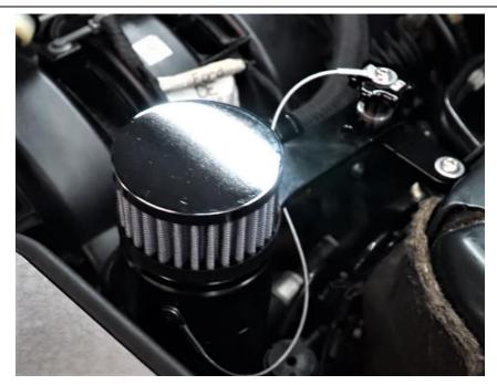
Install the catch can onto the bracket with the supplied knob (knob style may vary from photo).
