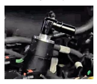
Remove the factory oil fill cap and install the UPR oil fill adapter. Mark where you want the fitting to face, remove the oil fill adapter from the valve cover, screw the fitting into the oil fill adapter and reinstall.
