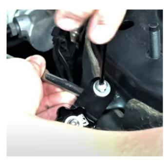
Using the supplied hardware, install the catch can bracket onto the driver side shock tower tab.
