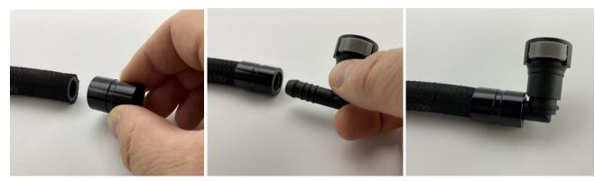
The hose included has one end left off so you can cut it to the length you need. Install the hose end cover, then lubricate the barbed fitting with a little engine oil and push it into the hose.
