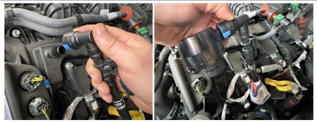
10 Release the VPS tube fitting on the driver side valve cover. To do so, just flip the tab on the side of the fitting. Rotate the fitting in the VPS tube 90 degrees so that it faces the front of the truck. Push the VPS tube fitting onto the UPR CSS male Plug N Play fitting.
