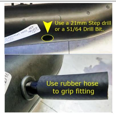
8 Drill the hole at the location marked, avoiding any seams. Push the supplied grommet into the tube and push or twist the fitting into the grommet. You can use a short section of rubber hose to help grip the fitting. Reinstall the turbo inlet tube. After installing the inlet pipe you can now connect the WOT line.
