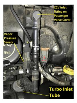
9 Locate the Crankcase Vent tube (CCV) on the driver side valve cover.
