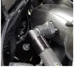
7 Remove the passenger side turbo inlet tube to prepare to drill and install the supplied grommet and fitting. The clamp on the coupler at the passenger turbo is easily accessed from the passenger front wheel well area.
