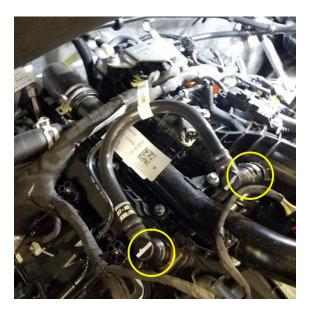
3. Locate the harness retaining stud on the top driver side of the fan shroud. Remove the Stud, and reinstall it through the catch can bracket to mount the catch can.
