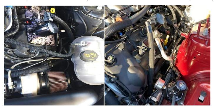
6. Install the Clean Side Separator (CSS) onto the driver side valve cover by lifting up on the collar and pushing it onto the driver side PCV fitting. Connect the hose from the CSS to the Quick Tap fitting on the turbo air filter. Sleeper kits will have a longer cut-to -length hose that you can route to the turbo filter under the car. Once you determine the length, install the hose end ferrule then the hose end fitting.
