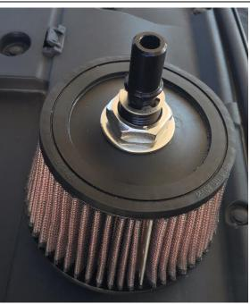
5. Install the supplied UPR Quick Tap Fitting into the driver side Tubo filter. Drill a 7/8 hole in the top of the filter. A step drill works best. Install the fitting from the inside of the filter and secure it with the washer, nut then clip.
