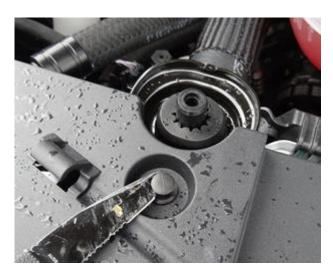
1. Remove the radiator cover by removing the plastic push pins. Use a knife, screwdriver, or pick to pull up the center of the pin, then remove the entire push pin assembly.
