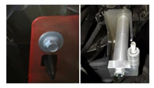
2. On the passenger side of the car, you will see a 10mm bolt that is just to the right of the radiator in the radiator support. Remove the bolt and install the UPR catch can bracket in it's place as shown.
