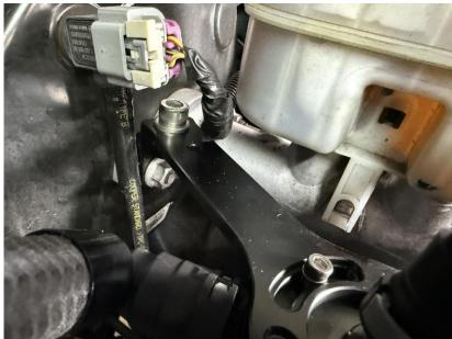
3. Remove the two connectors left behind hooked to the valve cover that vent to the airbox. Then install the new UPR Plug n Play™ Braided line to 'bridge' the fittings on the valve covers.
