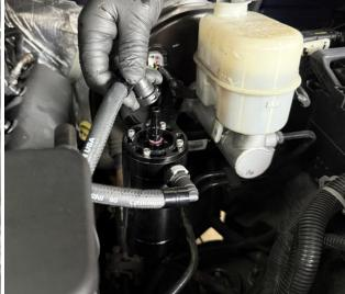
7. Install the provided Oil fill adapter fitting into the valve cover. The fitting can be installed and removed by inserting a 3/8 Allen wrench into the neck of the fitting.
