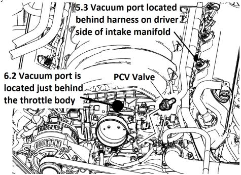
4. The 'Clean line' will be a 3/8 hose with a check valve in it. On a 5.3L engine, connect the hose to the fitting on the driver side of the intake manifold with the arrow on the check valve facing the manifold connection, away from catch can. (Behind injector above valve cover). On the 6.2L engine, connect the hose to the fitting just above the throttle body. Connect the other end to the side fitting on the catch can.
