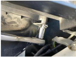
2. Locate the oval shaped hole in the frame on the driver side directly below the air inlet. Install the 90 degree mounting bracket to the frame with the supplied hardware. The bracket should be facing upwards. Install the catch can onto the bracket with the supplied hardware.
