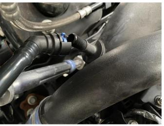
7. Connect male portion of the 3-way fitting into the CCV tube, and connect it to the turbo inlet tube as shown. The male end of the fitting should face the rear of the engine compartment.
