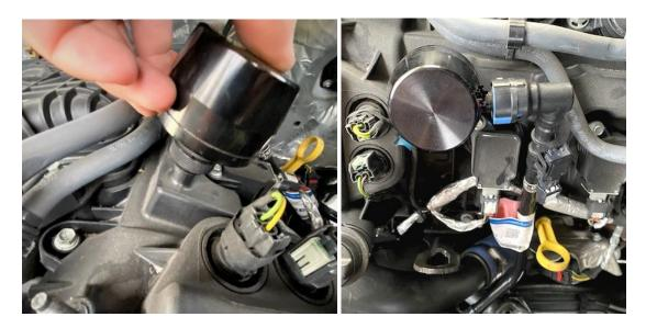
9. Connect the male end of the Wide Open Throttle (WOT) hose into the 3 way fitting. Connect the other end of the WOT hose to the catch can as shown. Make sure the arrow on the check valve is facing away from the catch can. (On some models it may be necessary to trim part of the engine cover to accommodate the new location of the driver side vent hose.)
