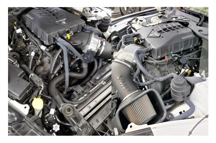
The Clean Side Separator will clip onto the driver side valve cover Crankcase Vent fitting. Connect the remaining hose from the Clean Side Separator to the Air inlet tube fitting.
