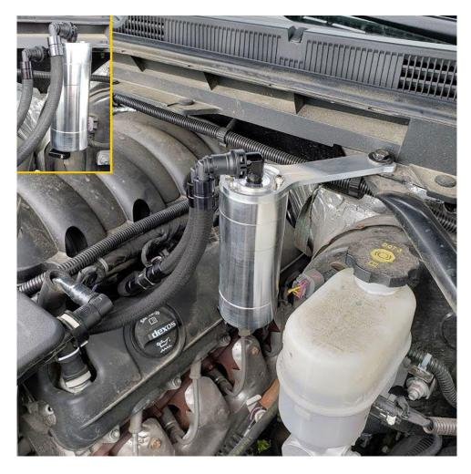
5. Double check and make sure all the Plug N Play fittings are clipped onto the OEM connections and the catch can. Periodically check the catch can every 1000 miles to get a feel for your truck's needs. Most will need the catch can to be emptied every 3-5000 miles. The containment cup on the catch can is able to be unscrewed for inspection.
