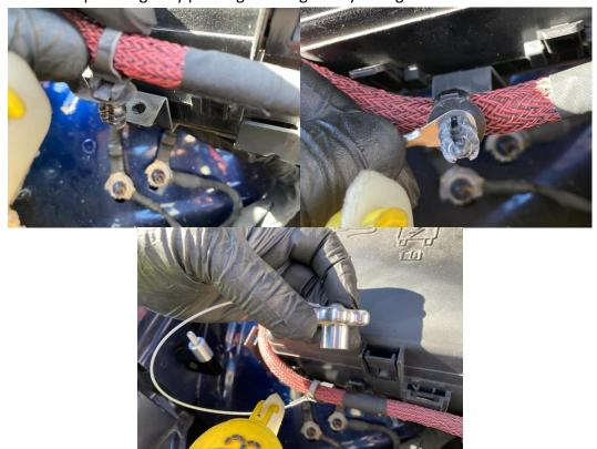
**4.** The UPR Catch Can kit comes with a quick release knob for the catch can mount. The lanyard on the knob prevents the knob from falling down into the unreachable parts of the engine compartment if it is dropped. Secure the lanyard by pulling the plastic harness clip up, pushing the lanyard eyelet on, and reinstalling the clip.
