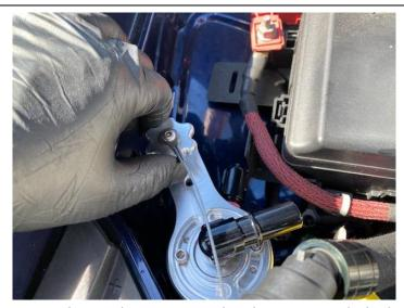
**5.** Set the Catch Can in place over the Fender Mount stud and secure it with the knob. Leave the knob slightly loose until the hoses are connected.
