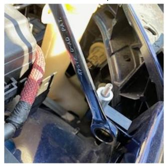
2. Locate the un used tab on the passenger inner fender well. Install the UPR Fender Mount bracket as shown. (For Export Models, you may need to move the sensor to the other side of the tab).
