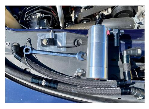
1. To install the UPR Single Valve Catch Can kit for the Hellcat/ Demon/ Redeye, you will need a 14mm wrench and a 5/32nds Allen key.
