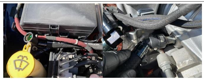
**3.** Remove the factory hose that connects the PCV valve on the passenger side valve cover to the vacuum port on the supercharger. The UPR vacuum hose will have a check valve in it. Route the hose under the fuse panel power cable so that the arrow on the check valve points towards the engine. Connect the hose at the supercharger by pushing the Plug N Play fitting on until it clicks.
