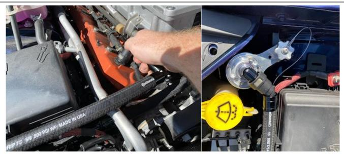
**7.** Connect the final hose to the PCV fitting on the valve cover. The hose will connect to the top fitting on the catch can. Tighten the UPR quick release knob, and reinstall the engine cover.
