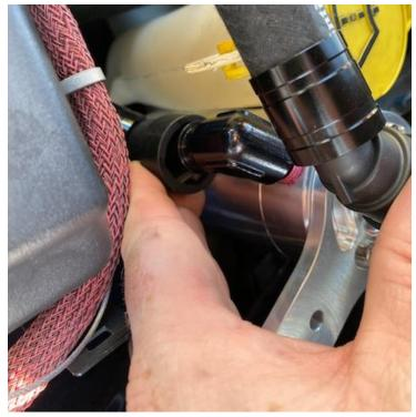
**6.** Connect the vacuum hose to the side fitting on the catch can. The UPR Plug N Play fittings will click when seated.
