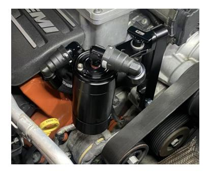
4. Mount the catch can to the bracket. Connect the PCV side hose to the top of the catch can by running the hose under the bracket as shown. Connect the remaining hose that is connected to the supercharger vacuum fitting to the side of the catch can.
