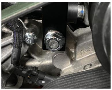
2. Mount the catch can bracket to the stud on the passenger side of the water pump with the supplied nut.
