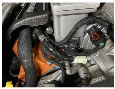
1. Locate the factory PCV hose that runs from the passenger side valve cover PCV fitting to the supercharger vacuum fitting and remove it. Save this hose in case you ever want to return the vehicle back to stock.
