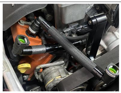
3. There are 2 hoses in the catch can kit. The hose with 90 degree fittings on both ends is the PCV side hose. The hose with a 90 and a straight fitting is the supercharger side (straight fitting connects to the supercharger vacuum fitting). Connect the hoses as shown before mounting the catch can.
