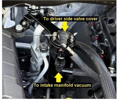
4. Install the "Dirty Side" PCV hose onto the top fitting of the catch can, and connect it to the driver side valve cover.
