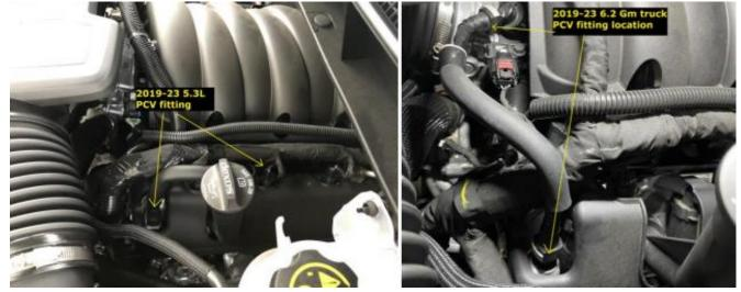
3. Install the 'Clean Side' hose from the side fitting on the catch canto the vacuum fitting on the intake manifold. (if you selected to add the Billet Pro Series check valve, the arrow on the check valve faces away from the catch can)
