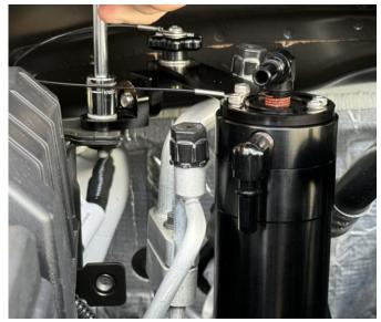
2. Remove the PCV hose connecting the driver's side valve cover to the vacuum port on intake manifold. Press the grey buttons on the fittings to release them.
