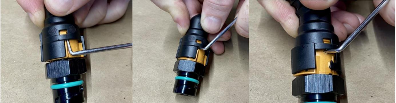
Now that you can see the 3 tangs, while applying upward pressure, use a pick or small screwdriver to release them.
