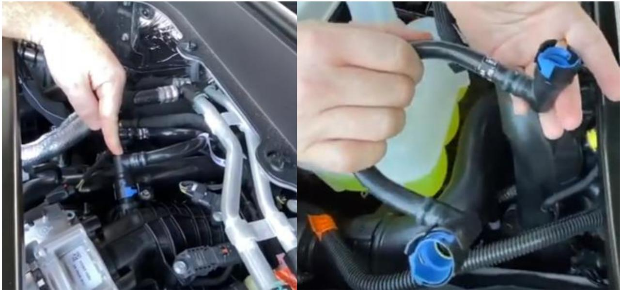
Locate the factory PCV hose that runs from the passenger valve cover to the intake manifold vacuum port.
