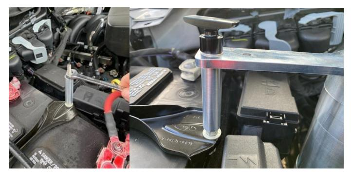
Install Threaded stud onto battery hold down stud and tighten. Install Catch Can with knob.
