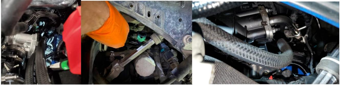
5. Position the coolant hoses back in place and reassemble the cover.
