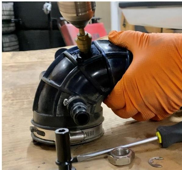
11. Disassemble the retainer clip, nut, and the washer from the Quick Tap fitting. Install the Quick tap fitting by pushing it up through the hole from the inside-out. Reinstall the washer, nut, then the retainer clip. Do not overtighten the nut. You can add a dab of RTV sealant to the base of the fitting before installing the washer if you made the hole a little too big.
