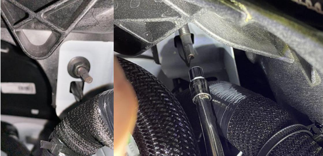
1. Looking toward the front of the engine compartment on the passenger side by the radiator, locate the stud and nut shown. Remove the factory stud, nut and washer pictured. This is where you will be installing your UPR fender mount catch can bracket. You will need a 5.5mm socket for the hex at the end of the stud, and a 12mm deep socket for the nut.
