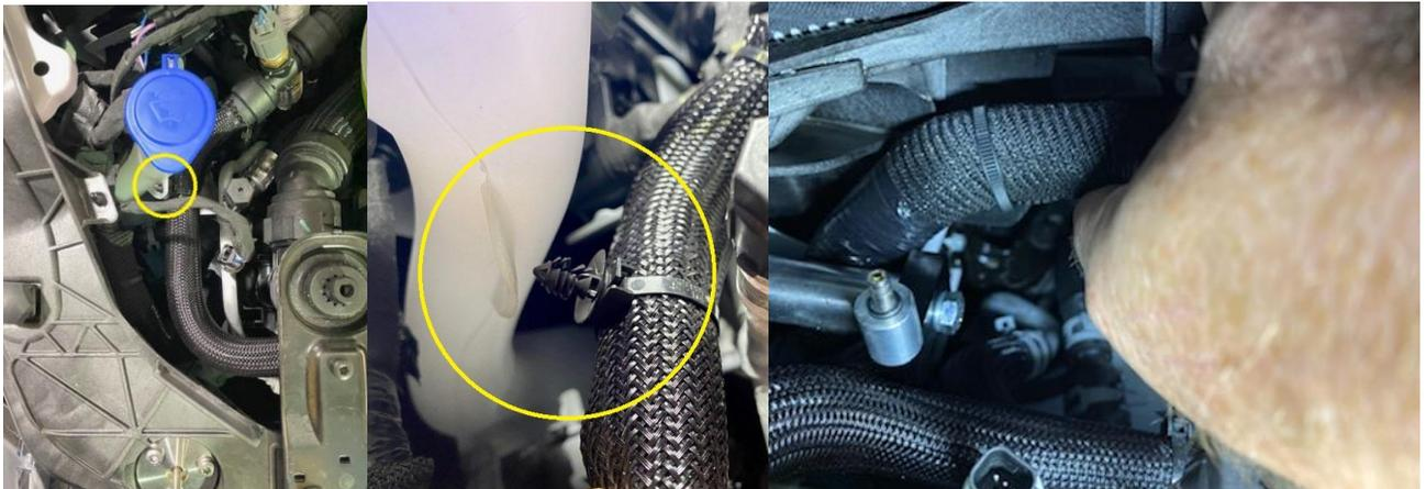
2. Remove the plastic retainer tree that attaches the coolant hose to the washer bottle. This will allow the hose to move and gain room for the catch can assembly. You may have to move the wiring harness over a little to allow the catch can to snugly drop in.
