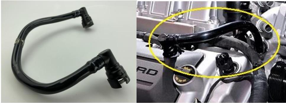
3. Remove the factory PCV hose that connects the PCV valve to the Vacuum port on the supercharger.
