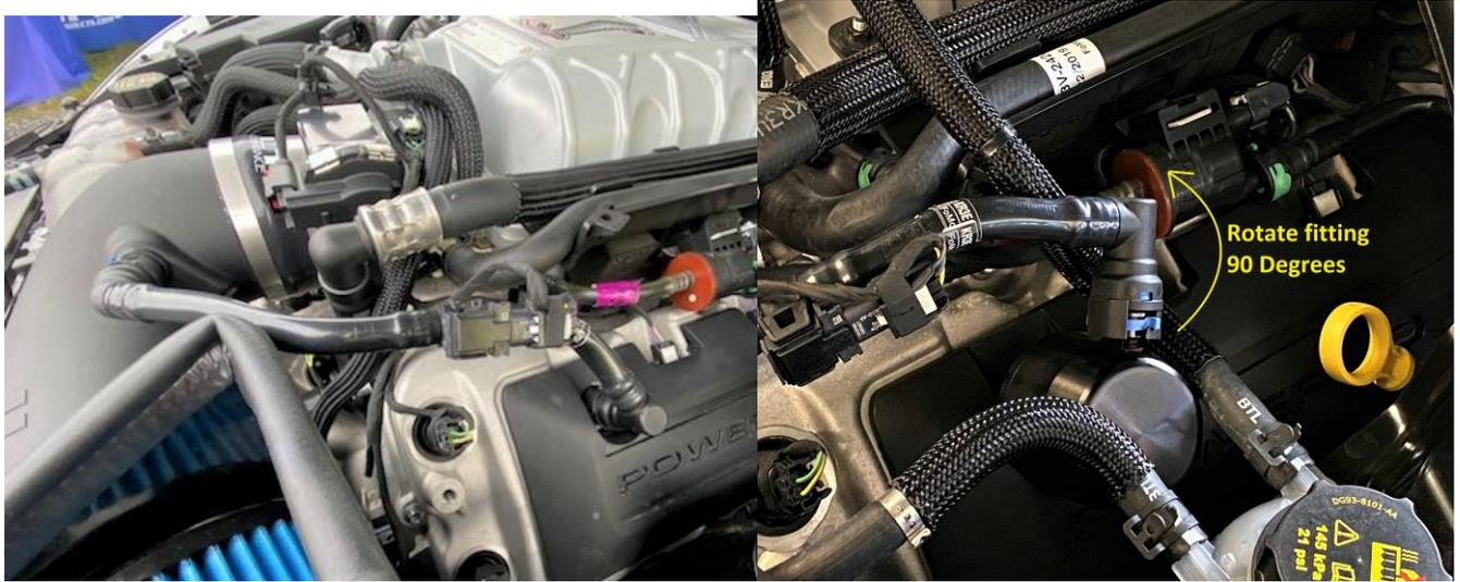
5. Locate the driver side crankcase vent tube. Disconnect the tube at the valve cover, but do not remove the tube. Rotate the fitting in the tube 90 degrees. Install the UPR Clean Side Separator by lifting up on the collar and pushing it onto the valve cover fitting until it clicks. Connect the crankcase vent tube to the CSS as shown.
