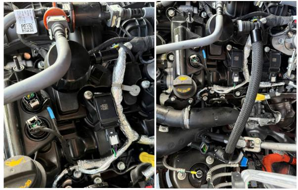
13. Install the CSS onto the driver side valve cover by lifting up on the collar, and pushing it onto the fitting until it clicks. The evap hose will be very close or may touch the CSS. This is normal. Install the CSS hose connecting the CSS to the 3 way fitting.
