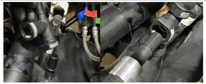
12. Install the 3-way Plug N Play Wide Open Throttle adapter fitting onto the driver side turbo inlet tube so that the female leg of the Tee is facing forward. Route the short hose (the Wide Open Throttle or WOT hose) from the catch can to the 3 way fitting. Connect the male fitting on the WOT hose from the catch can to the female fitting on the Tee.
