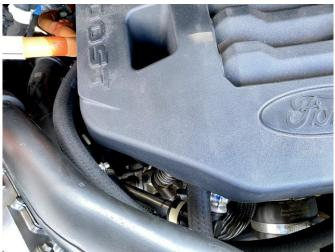
15. Reinstall the engine cover and tighten the 10mm nuts. Be sure the hoses clear the cover and do not interfere with other engine components.
