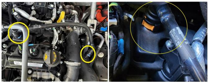
6. All 2024-up 3.5L Eco boost F150s we have seen no longer have the orange, non-quick release fitting on the driver side valve cover. (YAY!) If you have blue quick connect fittings, removing the driver side hose is as easy as the passenger side.
