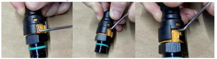
9. Another Method to remove the fitting is to separate the orange portion of the fitting from the outer cover. Using a pick or flat screwdriver, find the small orange 'window' on each side of the fitting. Slide the pick or screwdriver up between the black outer portion of the fitting and the orange inner portion. Pry up on each side to pop the outer portion off.
