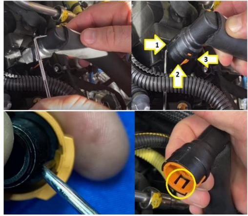
8. While holding the hose and pulling upward lightly, run the pick under the fitting to release all 3 tabs. If the fitting or tabs break, the fitting can be replaced with a standard UPR Plug and Play fittings P/N 2025-39 (straight), 2025-40 (90 degree) or 2025-41 (45 degree). Repeat the process to remove the fitting at the other end of the tube.
