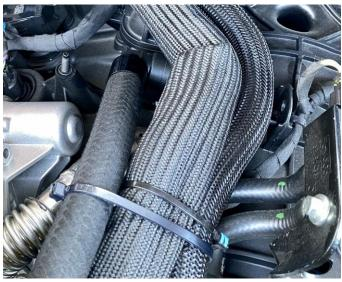
14. Secure the hoses to ensure they do not encounter any hazards like hot components, fans or belts. A good tip is to zip tie the vacuum hose along the coolant hoses on top of the intake manifold.
