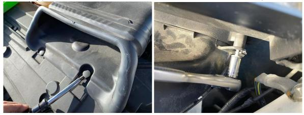
2. Locate the Square hole to the rear of the oval shaped hole on the flat portion of the frame on the driver side directly below the air inlet. Install the 90 degree mounting bracket to the frame with the supplied hardware as shown. The bracket should be facing upwards. Install the catch can onto the bracket with the supplied hardware. You can adjust the angle of the catch can by loosening the screws on the can and clock it into the best position.
