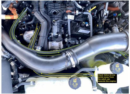
Find the longest hose in the kit with a check valve in it. Route the hose so that the arrow printed on the check valve faces away from the catch can, towards the engine. Connect the hose to the intake manifold vacuum port, and the other end to the outlet port that is furthest forward on the catch can. We found it easiest to route the PCV hose along the intake tubes going to the air box, and the vacuum hose forward and along the coolant bottle.
