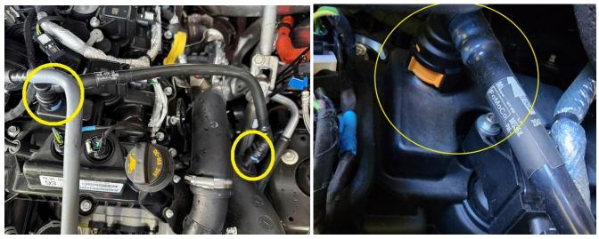
6. All 2024-up 3.5L Power boost F150s we have seen no longer have the orange, non-quick release fitting on the driver side valve cover. If you have blue quick connect fittings, removing the driver side hose is as easy as the passenger side.
