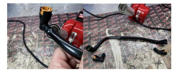
11. To replace the fittings on your factory CCV tube, use a heat gun or lighter to gently warm the plastic tube – do not melt or burn the tube. Pull the fitting out of the tube once it is warm, (Be careful, it will be HOT) and insert the new fitting into the tube while it is still warm. The tube will conform to the fitting as it cools. To assist, you can wrap a small zip tie around the tube ends while it cools. This is only needed if you want to return your truck to stock.
