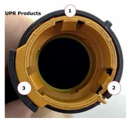
7. There are 3 little tabs securing the female end of the fitting onto the valve cover fitting. You can use a 90-degree pick or hook pick to release the fitting.
