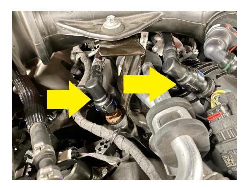
2. Locate the U shaped PCV hose that connects from the passenger side valve cover to the intake manifold. Remove it by releasing the quick release fittings.
