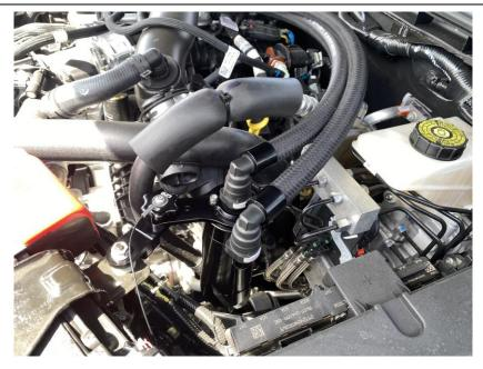
3. The top fitting on the catch can is the inlet from the PCV. Connect this hose to the PCV fitting on the passenger side valve cover. The side fitting will connect to the intake manifold. The arrow printed on the check valve in the hose connecting to the intake manifold must face away from the catch can.
