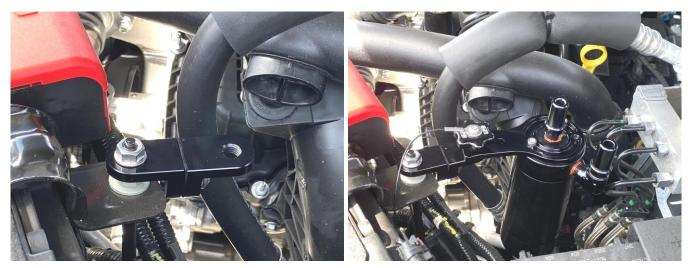
1. Install the bracket extension onto the rear battery tray stud. Install the UPR catch can using the supplied knob. You can adjust the position of the catch can with the brackets.
