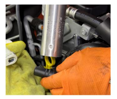
13. To replace the fitting on your factory CCV tube, use a heat gun or lighter to gently warm the plastic tube – do not melt or burn the tube. We covered the area under the fitting to protect the engine and components from the heat from the heat gun. Pull the fitting out of the tube once it is warm, (be careful, it will be hot) and insert the new supplied fitting into the tube while it is still warm. The tube will conform to the fitting as it cools.
