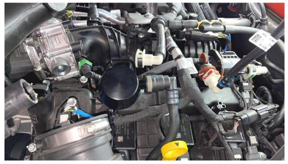
14. To install the Clean Side Separator, (CSS) pull up on the collar at the base of the CSS and push it down onto the CCV fitting on the valve cover. Once the CSS is installed fully onto the CCV fitting, the collar will click on to secure it. A little oil applied to the valve cover fitting can help the CSS to pop on smoothly. Rotate the fitting on the CCV tube and click it onto the CSS fitting.
