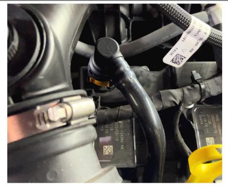
9. To install the Clean Side Separator (CSS), locate the crankcase vent fitting on the driver side valve cover. This fitting is not a quick release fitting. The following instructions will show how to remove and replace this fitting.
