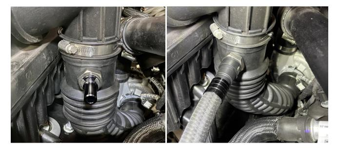
8. Reinstall the air inlet tube and connect the WOT hose connector.
