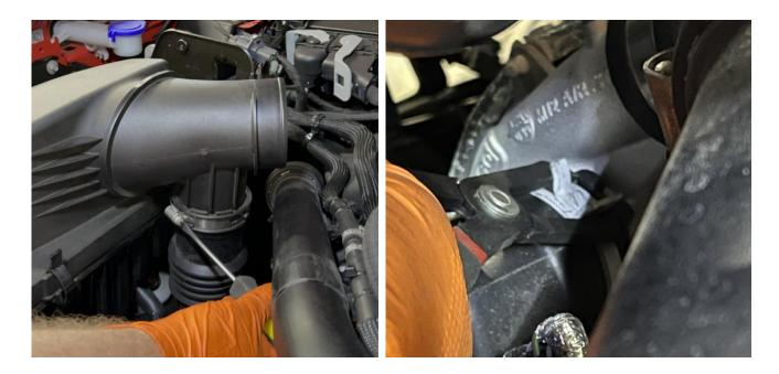
6. After marking the tube, remove the passenger side turbo inlet tube by loosening the hose clamp at the air box, and remove the air box cover. Use a pair of pliers to squeeze the clamp on the turbo inlet. When squeezed all the way, this clamp is designed to lock open which will aid re assembly.
