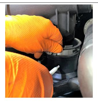
5. Mark the tube where the hose will comfortably reach. This is where you will drill a hole to install the UPR Quick Tap fitting.
