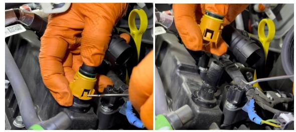
12. Once the outer cover of the fitting is off, while applying upward pressure, use a pick or small screwdriver to release the 3 tabs and remove it.
