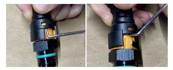
Here is a closer view of the orange windows on the fitting. Hook the pick under the black outer portion of the fitting below the orange window and pry up on each side.
