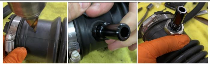
7. Use a 7/8 or 22mm drill bit to make a hole where you marked the tube for the UPR Plug and Play<sup>™</sup> Quick tap Fitting. (A step-drill bit works well). Install the fitting from the inside-out. Use the washer, retaining nut and clip to secure it. DO NOT OVERTIGHTEN the fitting or it can crack the tube. If you drilled the hole a little too big, don't panic. You can use a dab of automotive silicone sealant on the quick tap fitting
