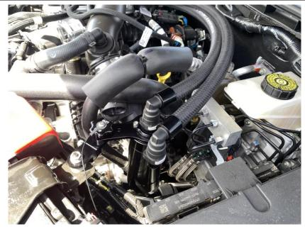
3. The top fitting on the catch can is the inlet from the PCV. Connect this hose to the PCV fitting on the passenger side valve cover. The side fitting will connect to the intake manifold. The arrow printed on the check valve in the hose connecting to the intake manifold must face away from the catch can.
