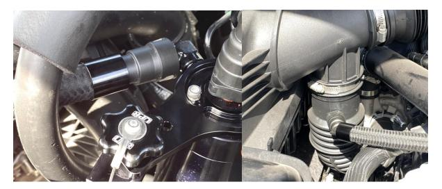
4. The third hose is the Wide Open Throttle hose (WOT). It will have a straight fitting on the catch can end and will have a check value in the length of the hose. Be sure the Arrow printed on the check value faces away from the catch can. Connect the hose to the catch can and route it towards the passenger side turbo inlet tube. It is the lower rubber tube connected to the air box.
