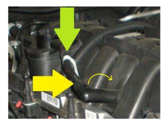
1. Remove the engine cover if equipped by pulling up on the cover. Remove the factory plastic PCV tube. Leave factory rubber PCV boots in place. Twist the 90-degree boot to face the front of the engine.
