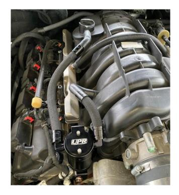
**5.** Install the barbed fitting and hose end cover onto the vacuum hose. Just like the PCV hose, insert it into the rubber boot, then onto the catch can.
