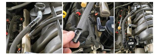
4. Install the barbed fitting and the billet hose end onto the catch can PCV hose. Push the fitting into the PCV boot. Before pushing the hose onto the catch can, install the billet hose end cover onto the hose and be sure it is routed so that it does not interfere with the engine cover fasteners. Once the hose is pushed onto the barbed fittings on the catch can, they will not come off.
