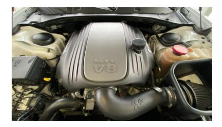
**6.** Double check the connections to make sure they are secure. Be sure the catch can mount is tight, and the containment cup is secure. Reinstall the engine cover. The UPR catch can is designed to fit under the factory cover. Some adjustment to the bracket mounting position may be necessary.
