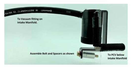
**2.** Assemble the Bolt and Spacers as shown. Remove the factory PCV hose. Install the UPR catch can bracket loosely in the top hole of the cylinder head. Push the PCV hose onto the PCV fitting. Position catch can and tighten the bracket. Install the Vacuum hose onto the vacuum fitting.
