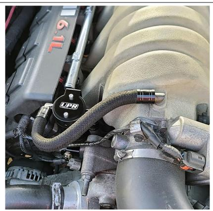
Always check and drain the catch can more often in winter / freezing weather. If the water/oil mixture in the catch can is allowed to freeze it will cause damage to the catch can and internal components. Any damage due to freezing is NOT WARRANTY. You must dispose of the liquid collected in the catch can properly (with used waste oil) properly according to your local laws.
