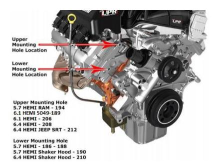
**1.** The UPR 6.1 Hemi catch can bracket will mount using the 'Upper' mounting hole in the passenger side cylinder head. See the above diagram to find the location.
