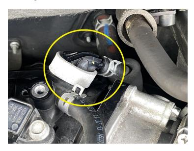
**4.** Install the barbed fitting into the hose and secure it with the factory clamp. Slide the hose end ferrule over the 3/8 hose, then push the hose over the exposed end of the barbed fitting. Route the other end of this hose to the smaller fitting on the catch can. Slide the hose end ferrule onto the hose, then push the hose onto the male fitting.
