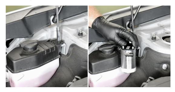
2. To access the PCV hoses, you will need to remove the engine cover. Lift up on the engine cover to remove it. Once the cover is removed, locate the vacuum manifold (grey plastic) that is just above the throttle body. Remove the single hose from the left side of the vacuum tree. This will allow you to move the vacuum tree out of the way for better access to the intake manifold PCV vacuum fitting.
