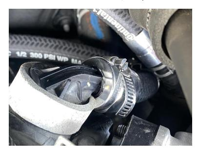
**6.** Go back over your connections to make sure they are secure. Secure the catch can by making sure the mounting bolt is tight. Do not over tighten the bolt, or damage to the coolant degas bottle can occur.
